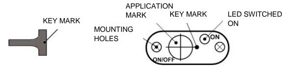
When applying the magnet to the key mark the green LED lights on permanently after a time lag of approximately 1 s and the electronic switch becomes switched on. Switching off takes place analogically, after renewed application of the magnet and another time lag of 1 s the green LED goes out and the system is switched off.
